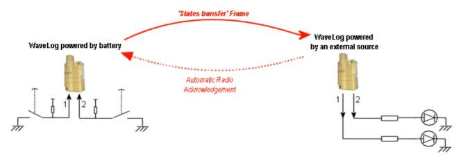
A rising edge on input 1 of WaveLog will be transfered on output 1 of receiver WaveLog. In the same way, the changes of states on inputs 2,3 and 4 will be transfered on outputs 2,3 and 4. WaveLog recipient has to acknowledge the received alarms frames.
